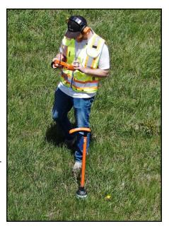
samples and tests, we identified a leak caused by a broken, abandoned service line that was leaching into a storm drain and into the customers' sump pump. Using the sound detected through the pavement, we alerted our distribution crew, and the leak was repaired!
