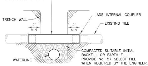
NOTE DO NOT BACKFILL UNTIL APPROVED BY ENGINEER.
