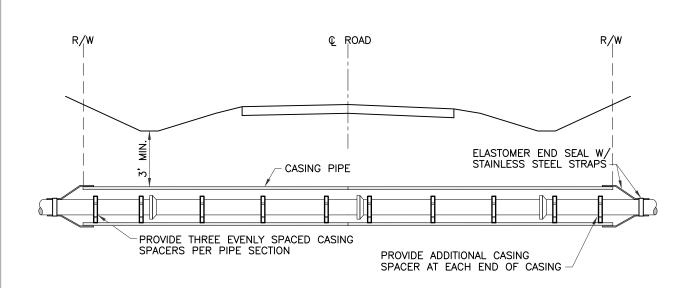
PROVIDE CASING PIPE FOR ALL ROAD CROSSINGS UNLESS OTHERWISE APPROVED BY DEL—CO. CASING PIPE SHALL BE STEEL PIPE WITH 0.375—INCH WALL THICKNESS, OR PVC C900 FOR WATER LINES 12—INCH DIAMETER OR LESS. CASINGS FOR WATER LINES LARGER THAN 12—INCH DIAMETER MAY BE AWWA C905. INSIDE DIAMETER OF THE CASING PIPE SHALL NOT EXCEED 3 INCHES OF THE OUTSIDE DIAMETER OF THE CARRIER PIPE AND CASING SPACERS.
